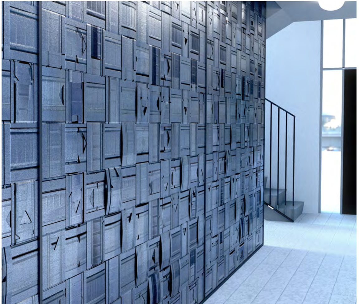
Figure 38/ Visualization of corridor with panels made from steel battens in a woven, sliding system.
